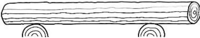
2. Select an approximate scribing distance This value depends on the log diameter and the carpenter's technique. For the present model calculation assume a preliminary scribing distance of 75 mm.
