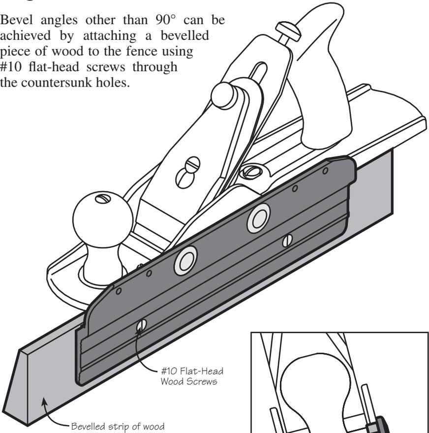
**Figure 5: Attaching bevelled piece of wood to inside face of fence to shoot bevelled edges.**
