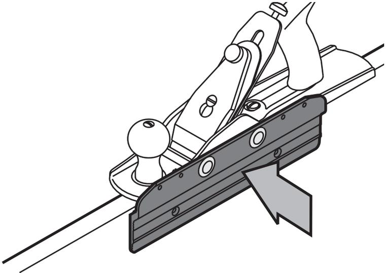
Figure 3: Fence held firmly against workpiece.
