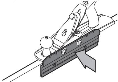
Figure 3: Fence held firmly against workpiece.
