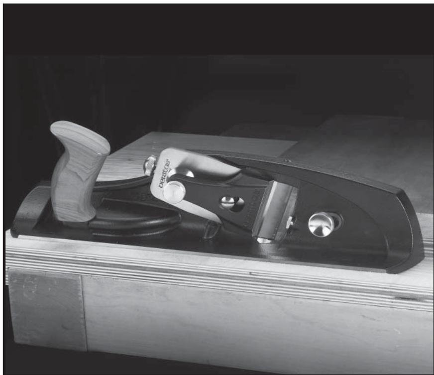
The Veritas® Shooting Plane is designed specifically to be used with a user-made shooting board to accurately trim and square the ends of workpieces. The plane weighs 7<sup>3</sup>/<sub>4</sub> lb so that it will have the momentum to easily cut through end grain. The body is just under 16" long and the base surface is 2<sup>1</sup>/<sub>8</sub>" wide. This plane is compatible with the Stanley #52 chute board.
